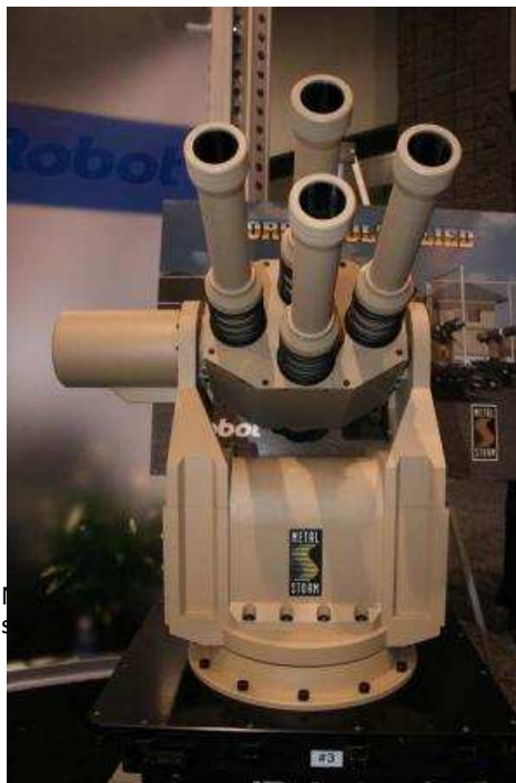
Metal Storm prototype grenade launch system (Source: Marine Corps Times)
